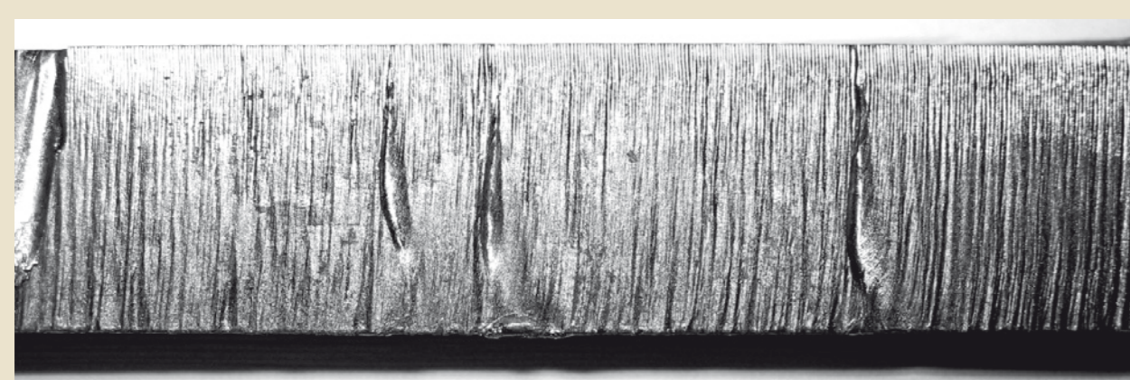
Example of how material quality can affect cut quality - oxygen cutting of low grade mild steel.
