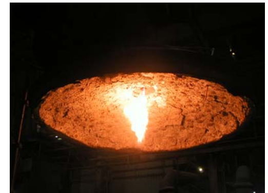
Ladle preheating at ACERINOX
