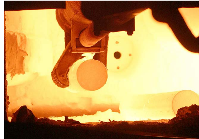
Rotary hearth furnace at ArcelorMittal Shelby, all equipped with flameless oxyfuel
