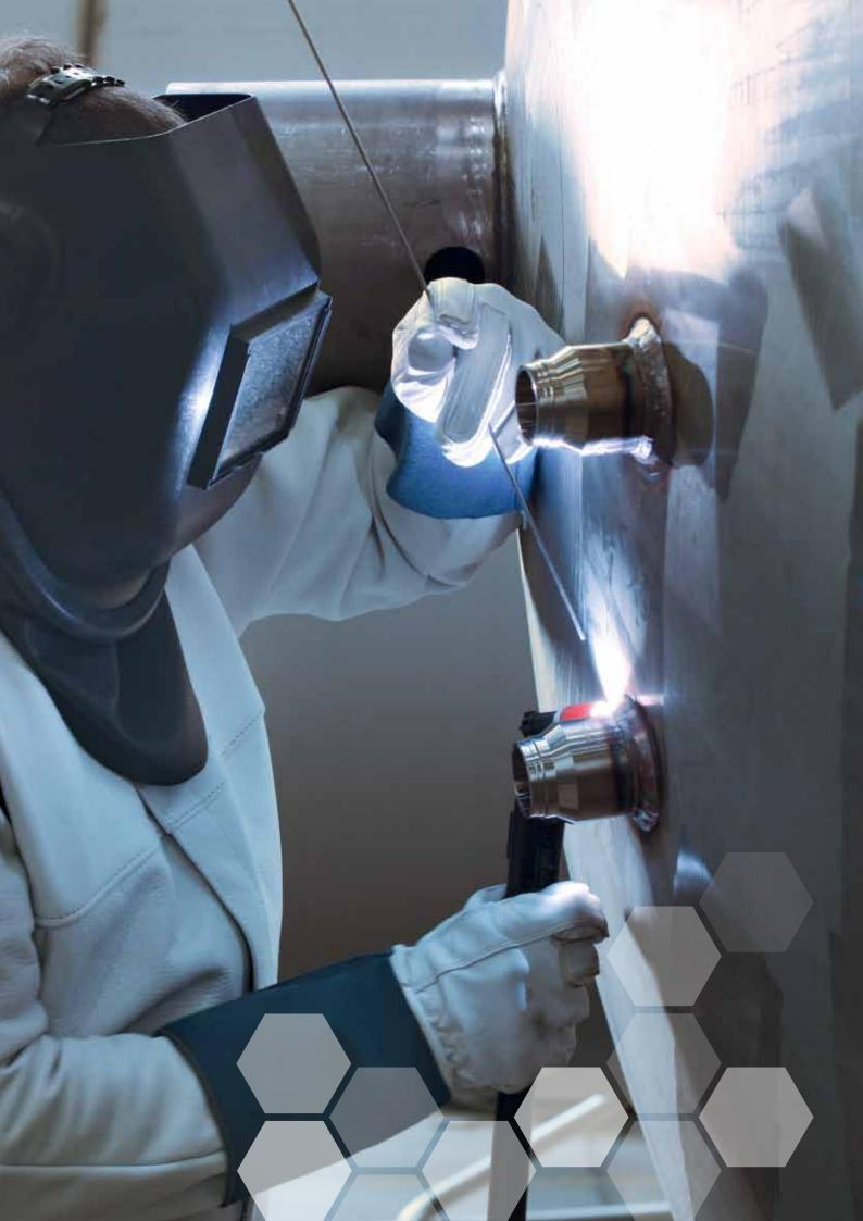
Stainless steel is usually defined as an iron-chromium alloy, containing at least 11 % chromium. Often containing other elements such as silicon, manganese, nickel, molybdenum, titanium and niobium, it is most widely used as corrosion resistant engineering material and it is used in applications where aggressive environments or elevated temperatures are prevalent.
