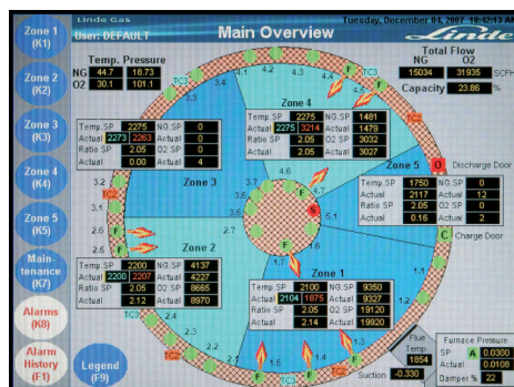
After revised heating profile the heating zones changed, two flue gas exits were closed and active pressure control implemented. Flameless oxyfuel has resulted in improved process yield with more uniform heating and reduced scale formation.
