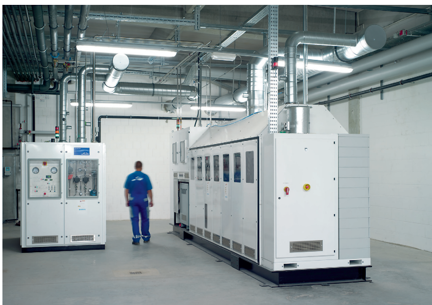
Fig 3. On-site generation of fluorine
