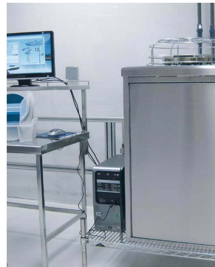
Atomic layer deposition system for 200 mm wafers inside Class 1000 cleanroom
