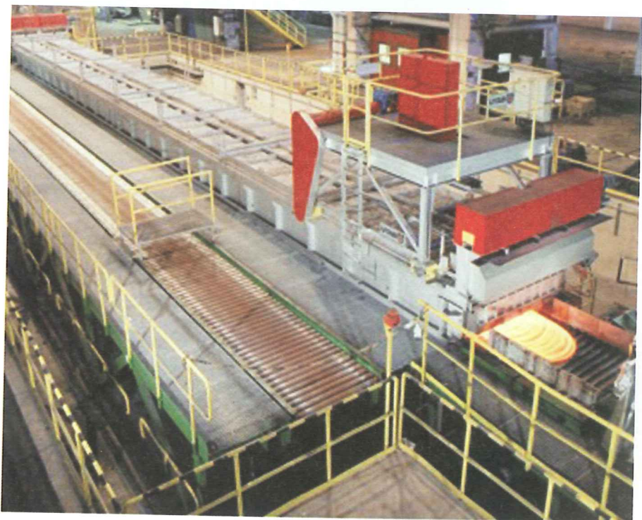
The Direct Solution Treatment furnace at Fagersta Stainless. Note that it can be shifted sideways to allow the roller table on the left to replace the furnace in the line.
